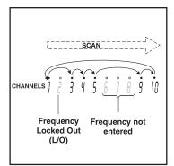
The scanner skips any unprogrammed channels, and locked out channels.
